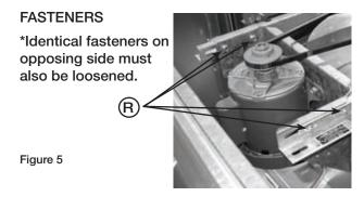
9. Belt tension should be adjusted to allow ½4 in. (0.397 mm) of deflection per inch of belt span. For example, a 15 in. (381 mm) belt span should have ½4 in. (0.234 mm) (or about ¼ in. (6 mm)) of deflection with moderate thumb pressure at mid-point between pulleys, see Figure 6.
